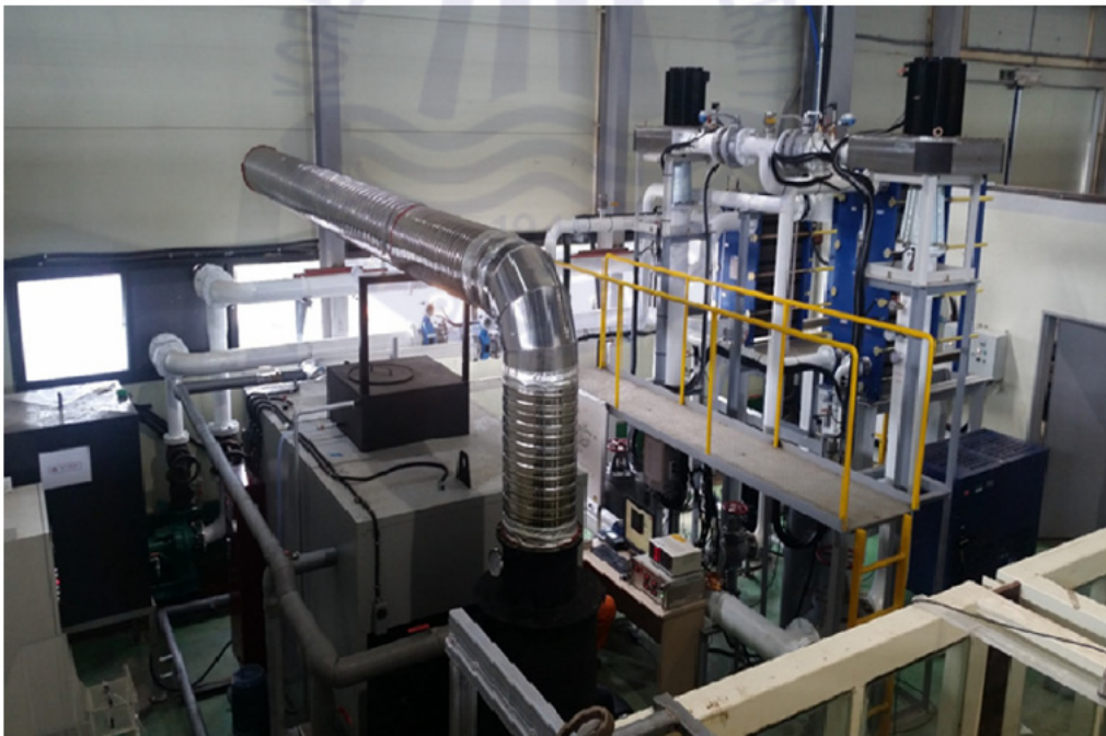
Fig. 7 Photograph of the experimental equipment for an organic Rankine cycle (Kim et al., 2019b)
