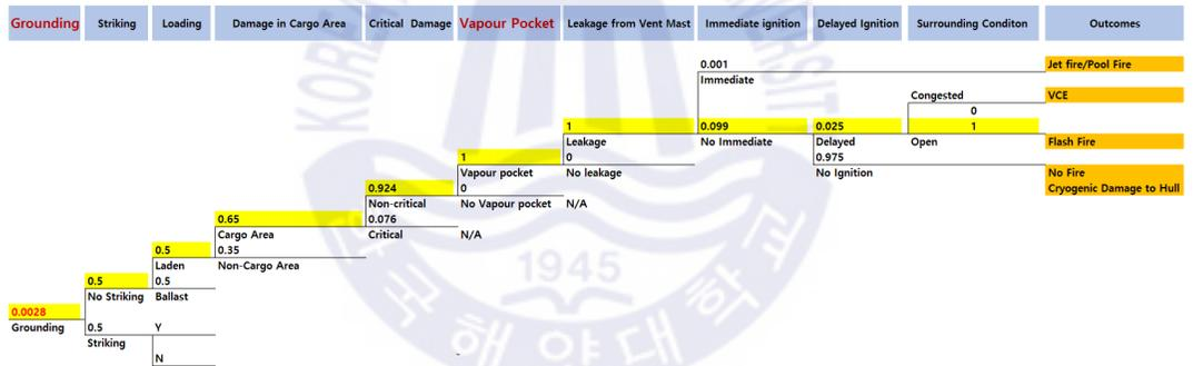
Figure 10 Event tree for grounding – vapour pocket
