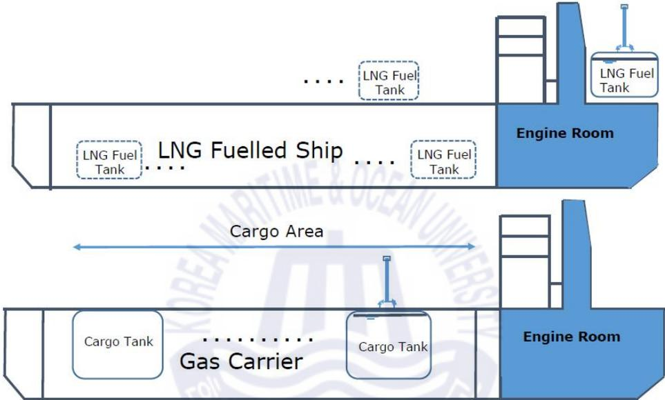
Figure 4 Brief arrangements of LNG fuelled ship and LNG carrier
