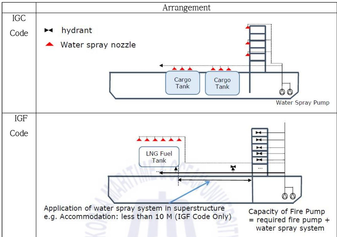
The IGC Code stipulates that exposed boundaries facing the cargo area, such as deckhouses and bulkheads of superstructures, should be covered by the water spray system. Besides, various other areas to be protected by the system are defined in the IGC Code 11.3.1 (IMO 2014c).
