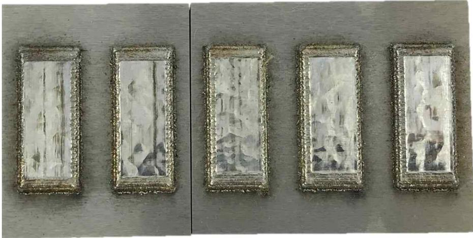
Fig. 34. UNSM treated DEDED 316L samples with optimized condition
