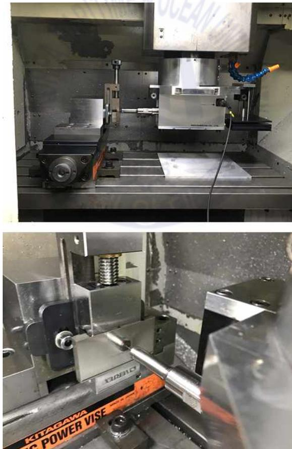
Fig. 4. Ultrasonic nanocrystal surface modification(UNSM) device
