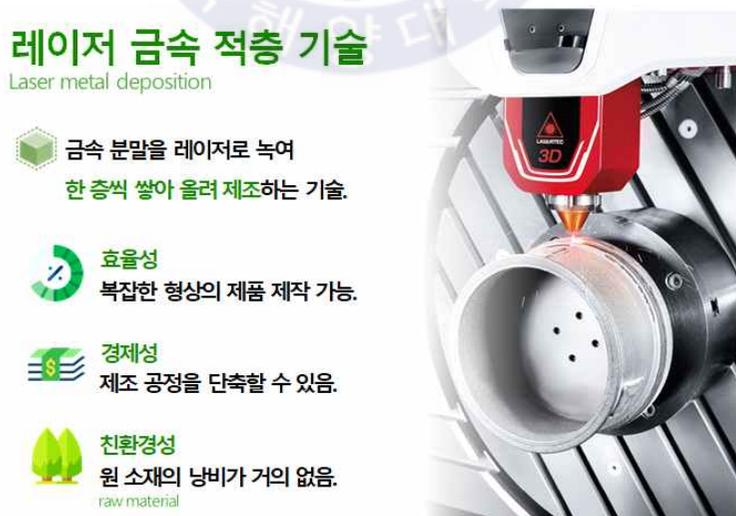
Fig. 1. Laser metal deposition
