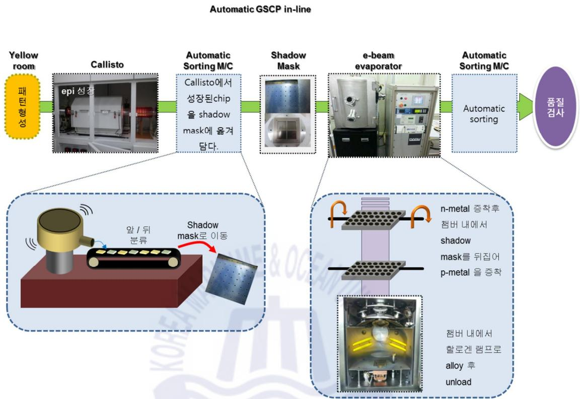
Fig. 31 Model of automation concept of HVPE GSCP vertical LED proposed in this paper
