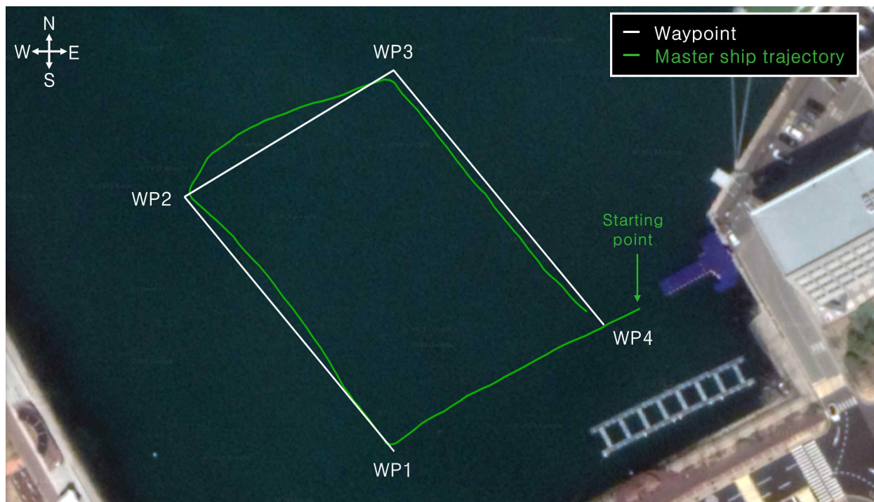
Fig. 3.15 Master ship trajectory during rudder control algorithm test
