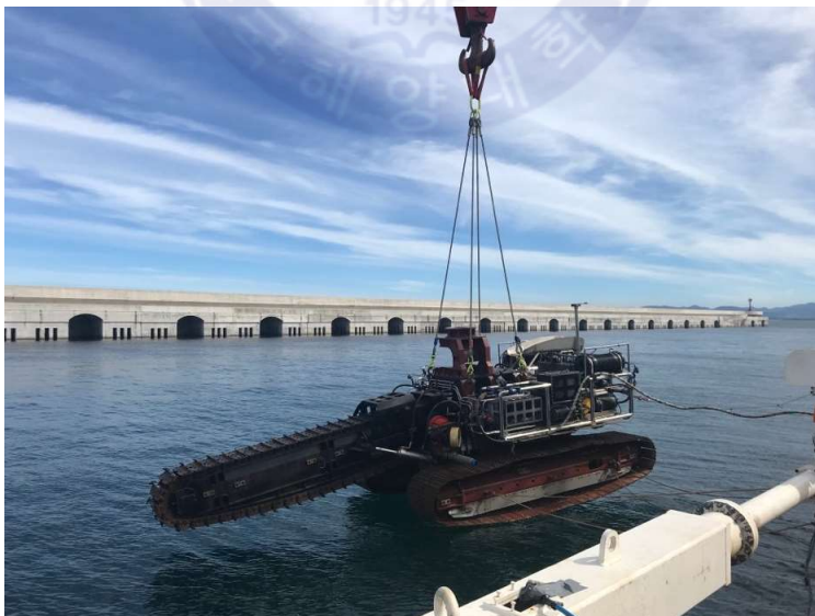
Fig. 5.4 Launching underwater track robot
