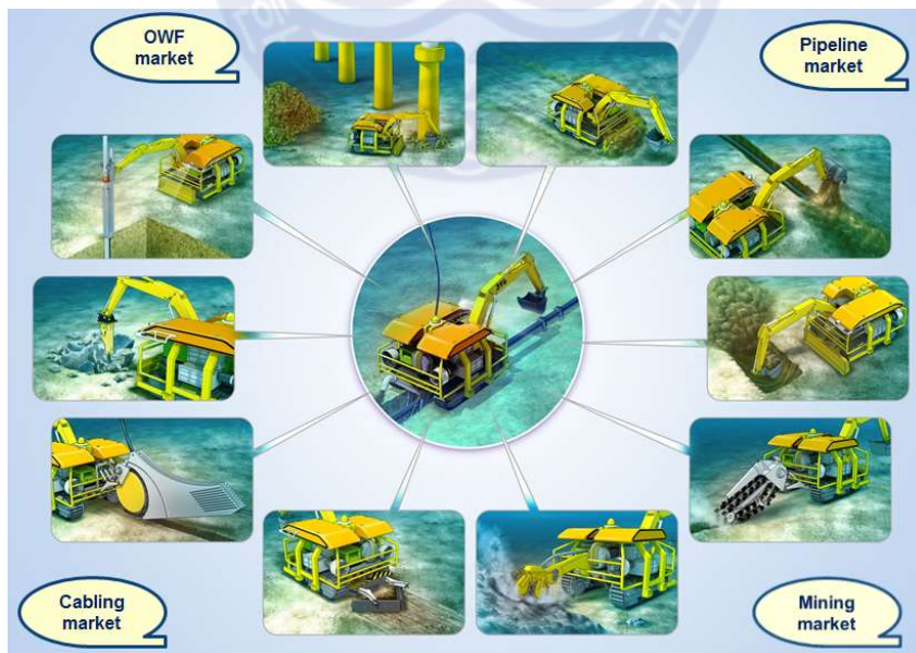
Fig. 1.2 Types and applications of underwater track robots
