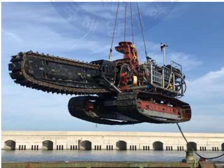
Fig. 5.1 Commercial trenching UTR
