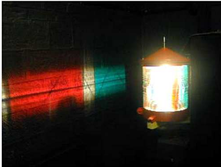
Fig. 42 Single light source sector light with drum lens
