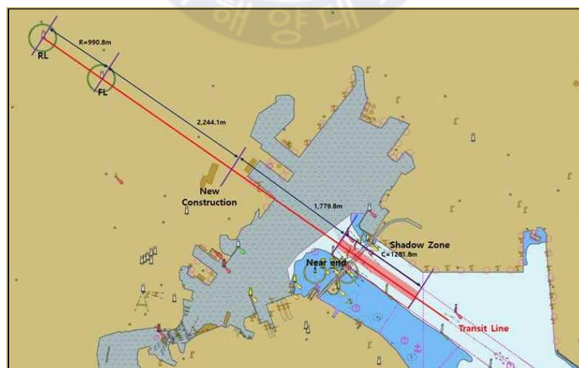
Fig. 68 Blind zone of Busan north port Leading Light(ground view)
