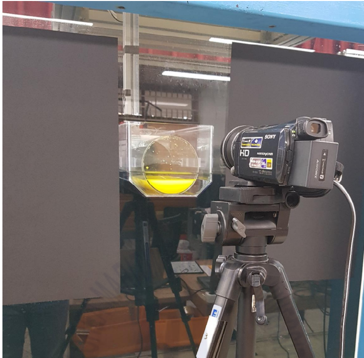
Fig. 18 Scale model test set up to research inner flow
