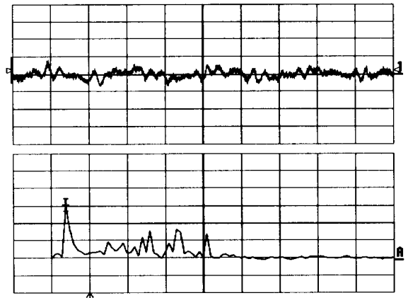
Ch.1: Discharge signal [ 2 mV/div, 10 us/div] Ch.A: FFT result [100 uV/div, 100 kHz/div]
