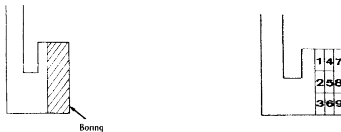
Fig.3 A typical repair welding method for the o-ring seat of diesel engines
