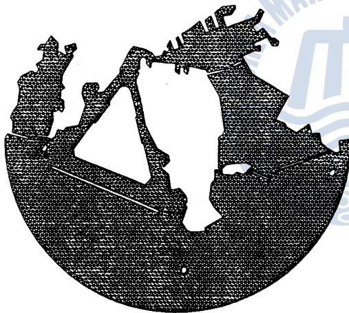
Fig. 6 Discretization of the artificial island project of Pusan harbor with triangular elements (4687 nodes and 8527 elements)
