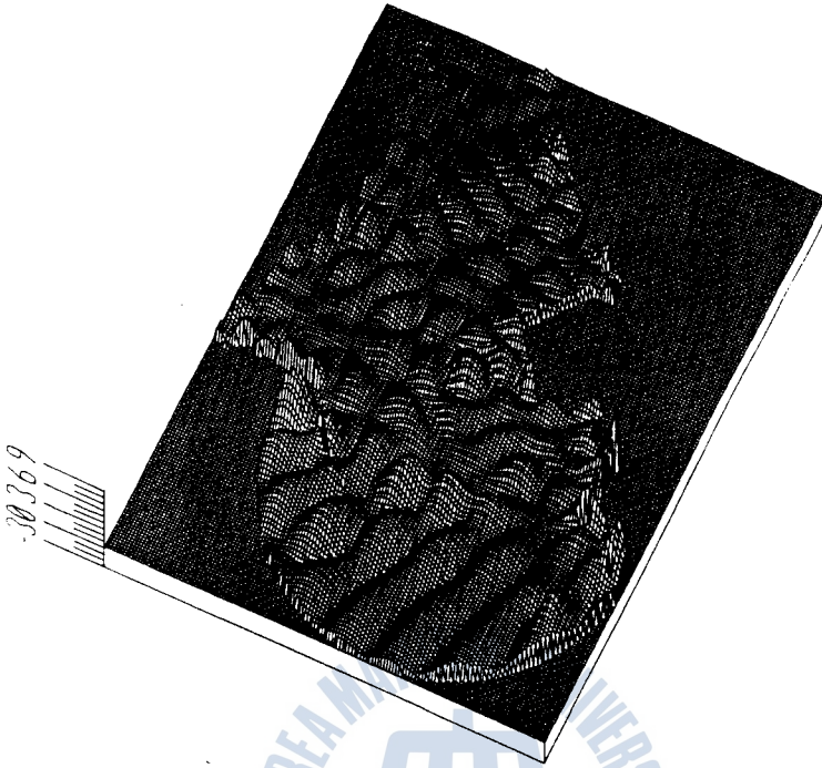
Fig. 13 Surface Pattern for Pusan Harbor (60sec, N50°E direction, K_r=0.9 , \beta=0.0 , open end)
