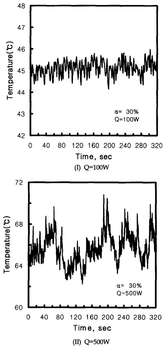
Fig. 5 Temperature variations of adiabatic section
