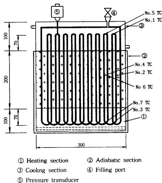
Fig. 3 A drawing of self oscillating heat pipe
