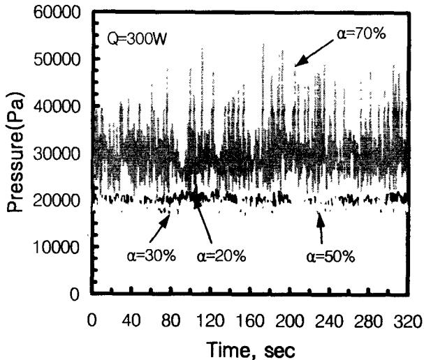
Fig. 8 Variation of pressure according to fill charge ratio
