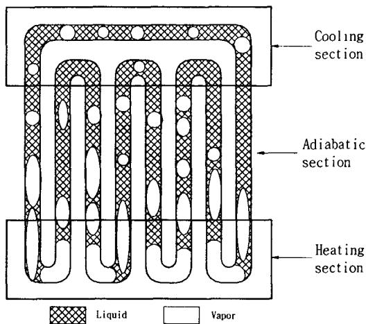
Fig. 1 Structure of self oscillating heat pipe
