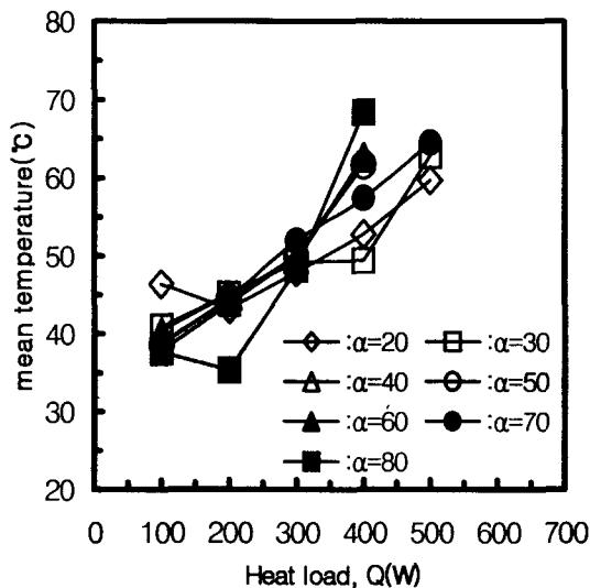
Fig. 6 Mean temperatures of adiabatic section
