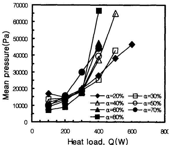
Fig. 9 Mean pressure on heat loads
