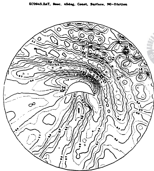
Fig. 4.6 Contour Wave Height Amplification Factor around an Emerged Semi-Circle Structure(9sec, 45° Direction, \beta=0.0 )
