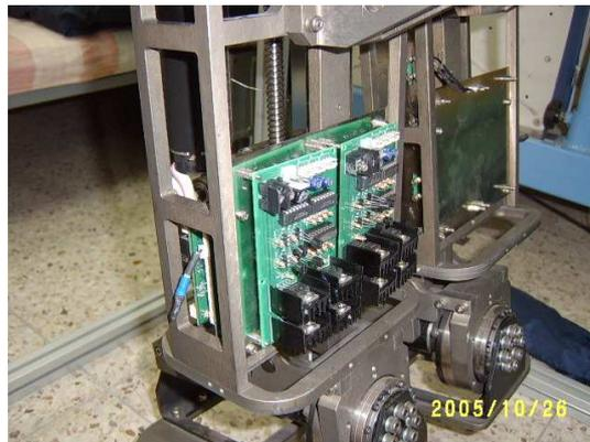
Fig. 2.14 Side view of the ankle actuator
