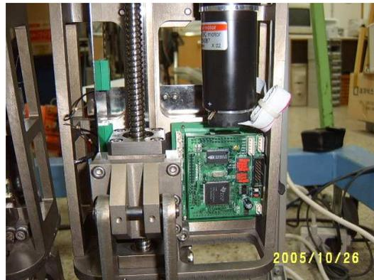
Fig. 2.13 Front view of the ankle actuator
