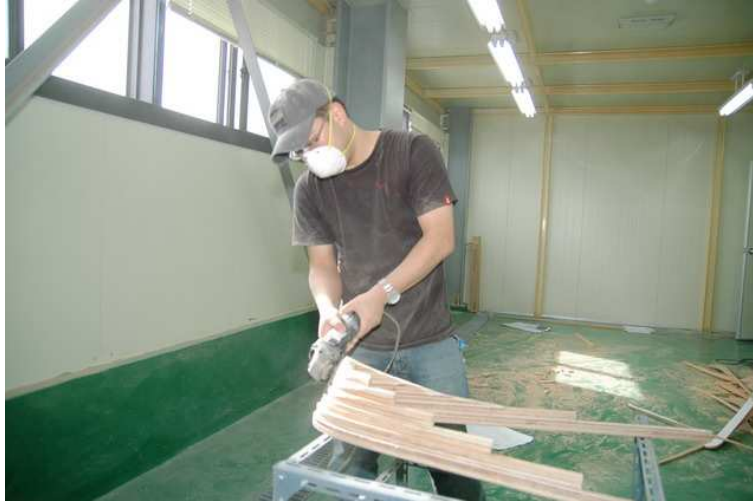
Fig. 53 Milling the kit parts from drawings for a canoe #7
