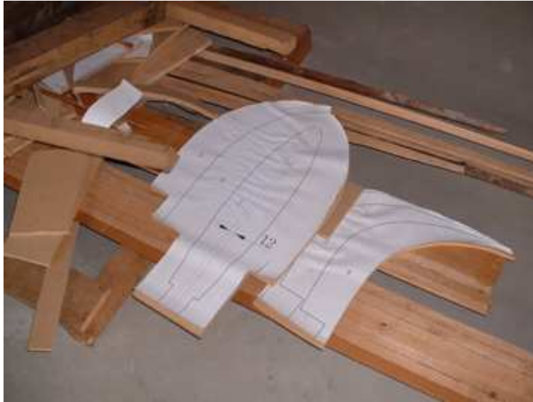
Fig. 9 Preparing the lines by the design of a canoe
