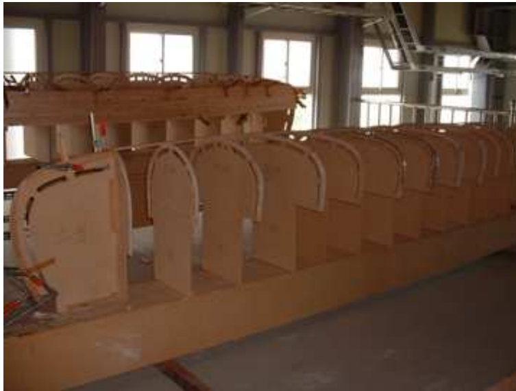
Fig. 10 Building the strongback for support the whole shape of a canoe
