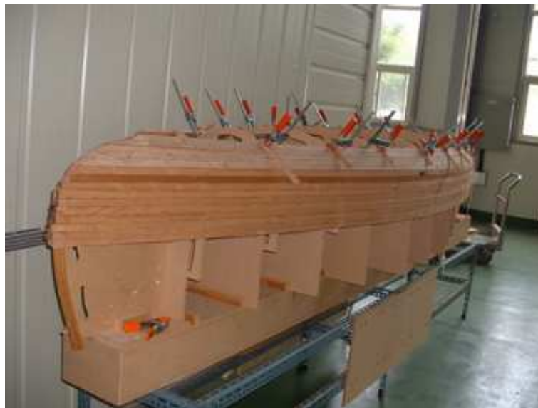
Fig. 12 Connecting strips over the strongback
