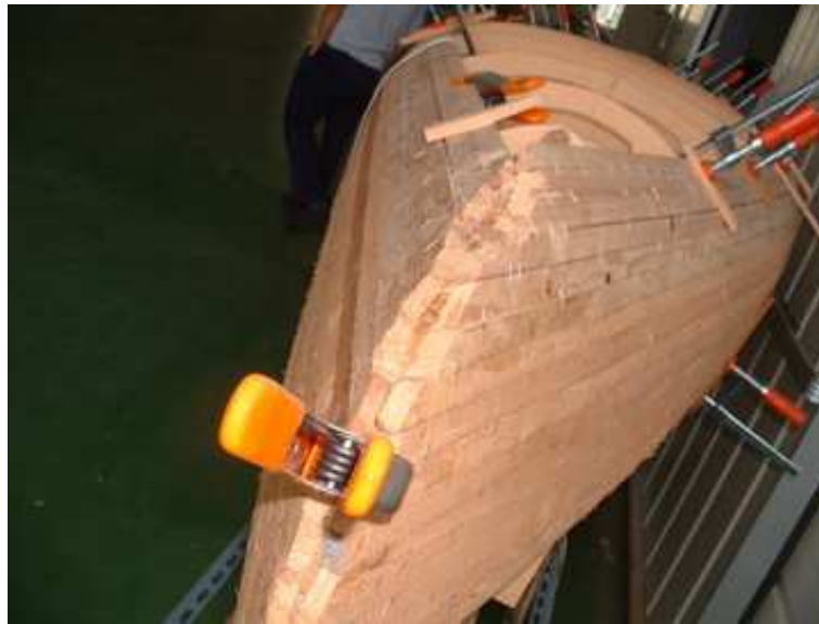
Fig. 11 Supporting for the bonding positions
