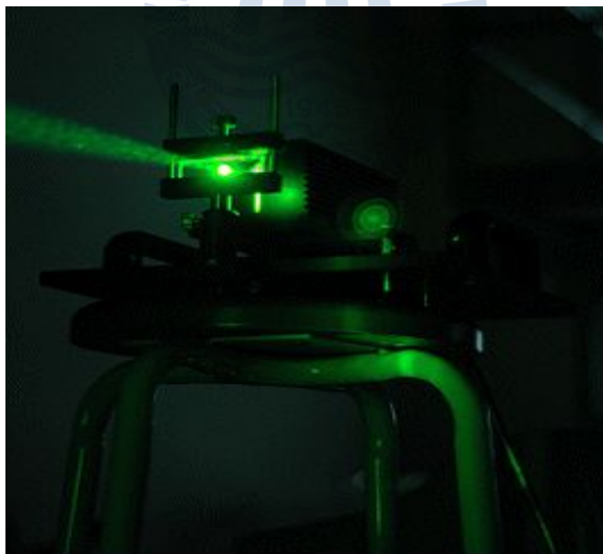
Fig. 10 Generated laser sheet PIV(Particle Image Velocimetry) analysis equipment
