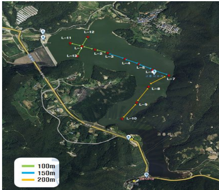
Fig. 37 Sampling point of test bed
