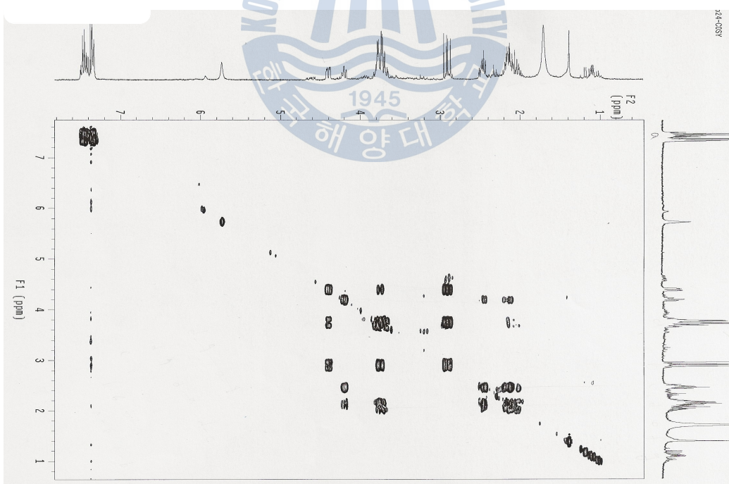
Fig. 19. COSY spectrum of compound 2 in \text{CDCl}_3 .
