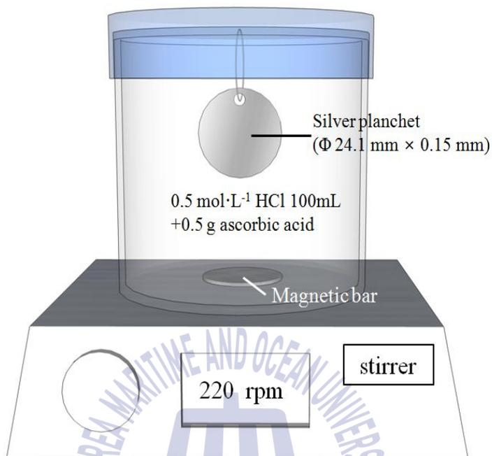
**Fig. 3** Spontaneous plating set for  $^{210}\text{Po}$  onto an Ag planchet.
