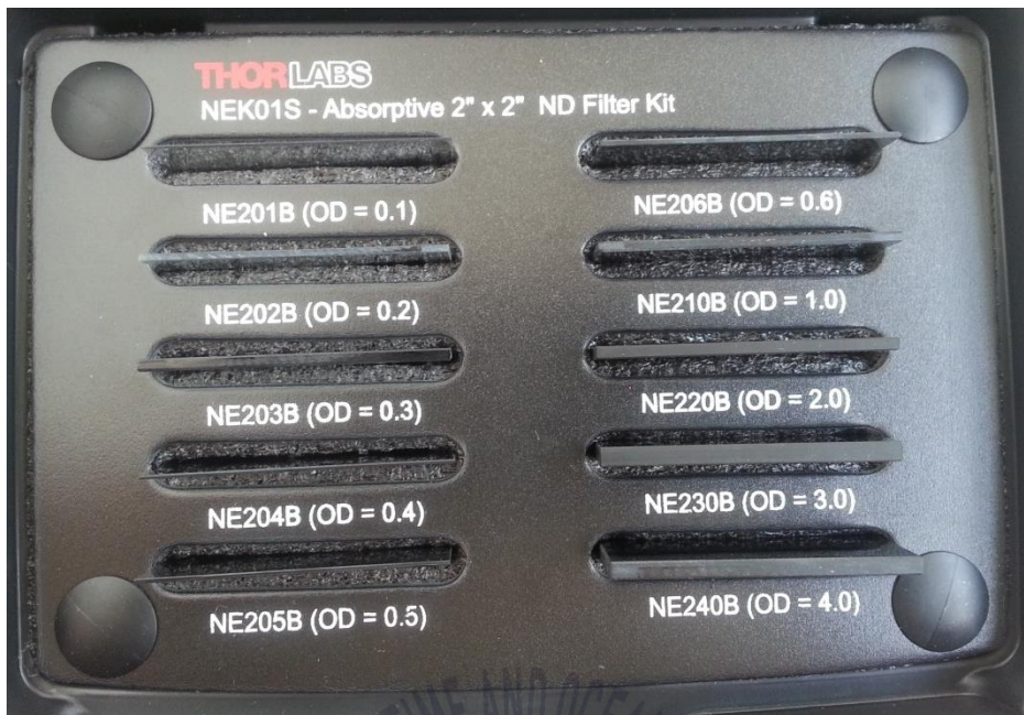
Fig. 8 Absorptive neutral density filter (optical density from 0.1 to 4.0)
