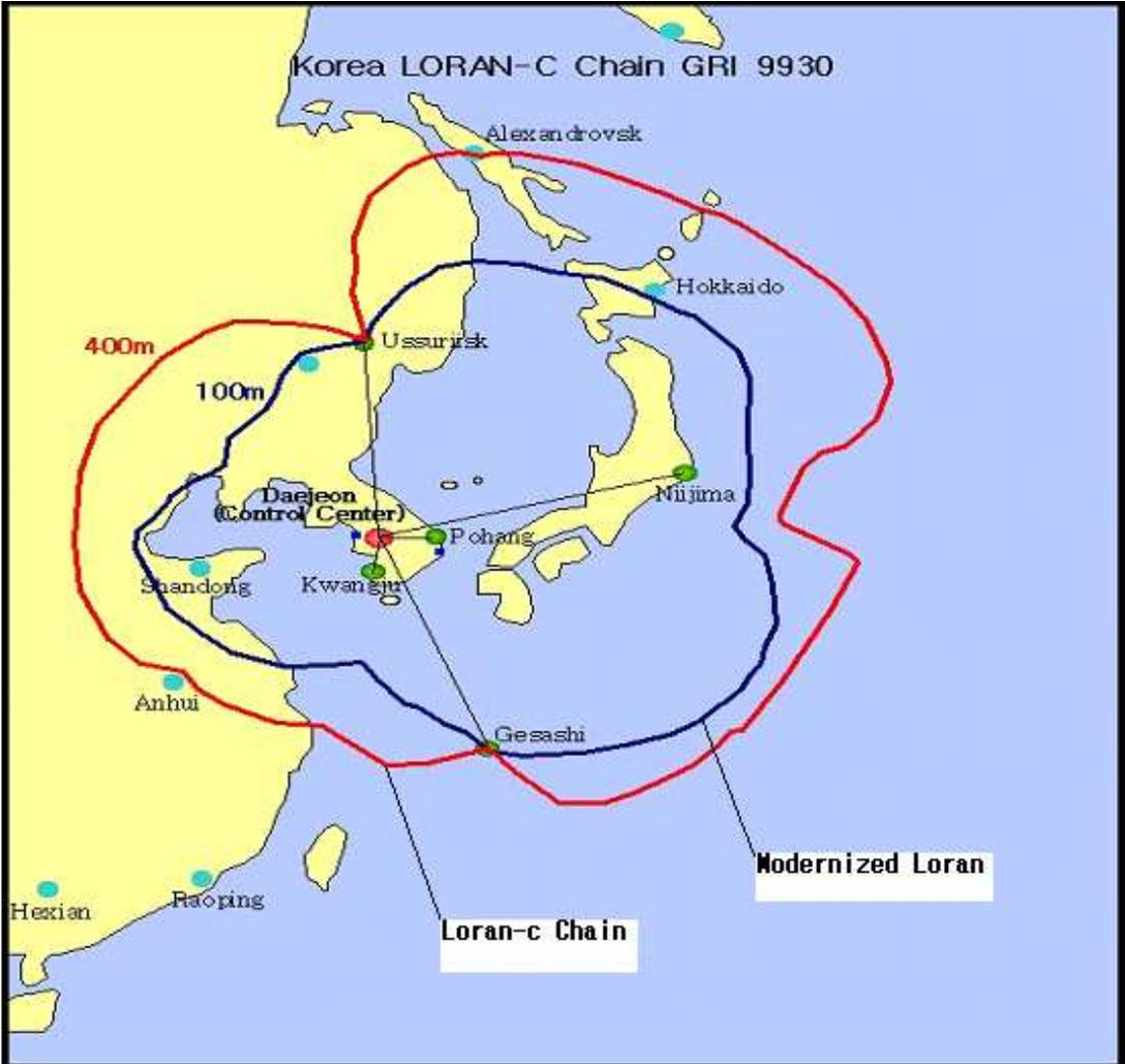
Fig. 3-16 Korea Loran-C and Modernized Loran Chains
