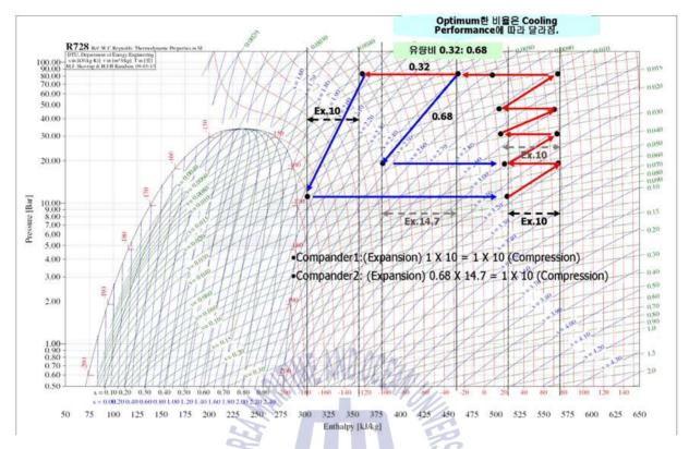
[Fig. 5.12] Mollier Diagram(P-H Diagram) of N<sub>2</sub> Expander Cycle
