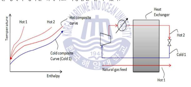
[Fig. 3.13] SMR (Single Mixed Refrigerant) Cycle
