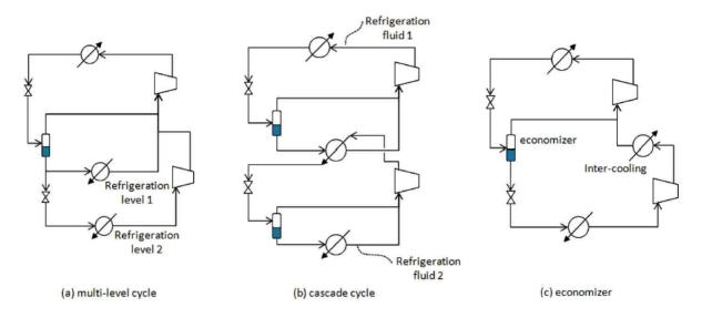
[Fig. 3.2] Structural Evolution of a Simple Refrigeration Cycle
