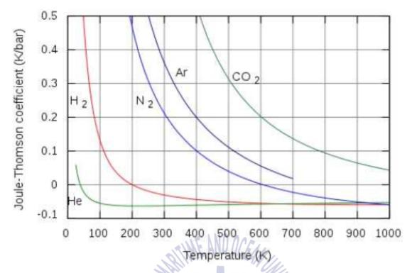
[Fig. 3.7] Joule-Thomson Coefficient Alteration of Various Gases
