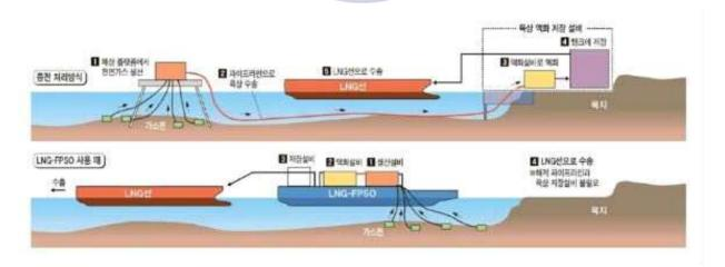
[Fig. 2.2] Onshore LNG Plant & Offshore LNG-FPSO
