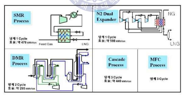
[Fig. 2.6] Natural Gas Liquefaction Process for LNG-FPSO
