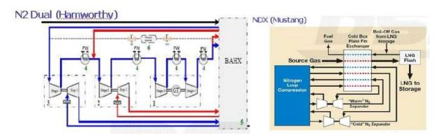
[Fig. 4.3] N2 Dual Expander Process
