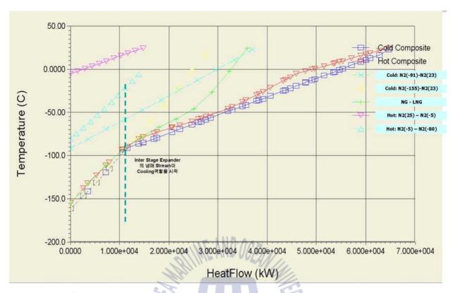
[Fig. 5.13] Temperature Alteration of N<sub>2</sub> Expander Cycle
