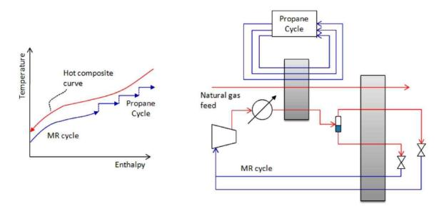
[Fig. 3.14] C<sub>3</sub>MR (Propane-Precooled Mixed Refrigerant) Cycle
