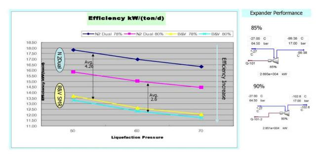
[Fig. 5.14] Efficiency Comparison of SMR Cycle vs N2 Expander Cycle
