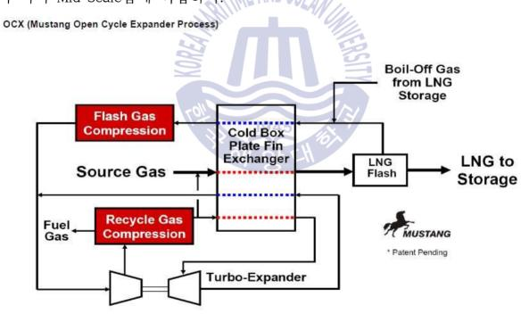
[Fig. 4.4] OCX(Open Cycle Expander) Process
