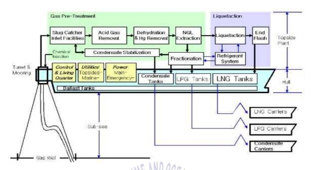
[Fig. 2.5] Process Flow Chart of LNG-FPSO
