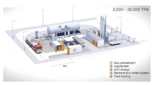
[Fig. 5.2] Mini Scale Liquefaction Plants
