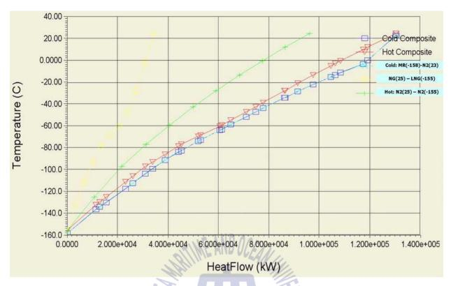
[Fig. 5.11] Temperature Alteration of SMR Cycle
