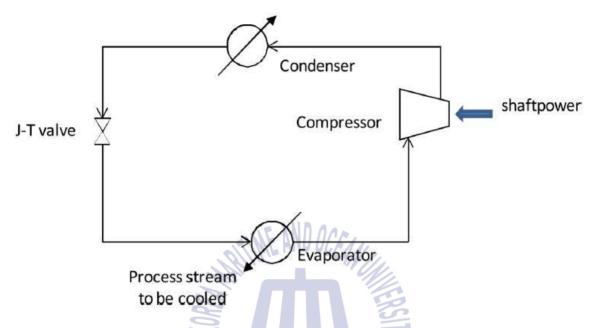
[Fig. 3.1] A Simple Refrigeration Cycle
