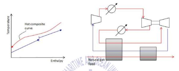
[Fig. 3.18] Nitrogen Expander Cycle
