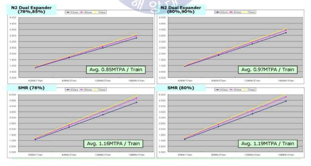
[Fig. 5.15] Production Comparison of SMR Cycle vs N<sub>2</sub> Expander Cycle
