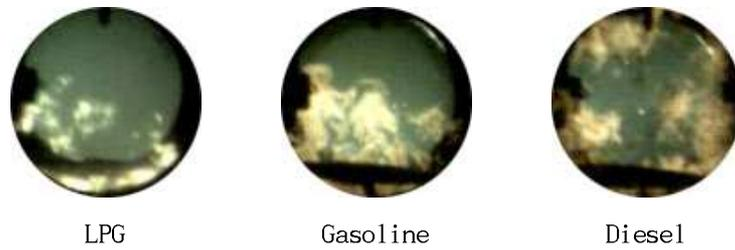
Fig. 3.60 Flames just before termination at trap pressure of 0.7MPa
