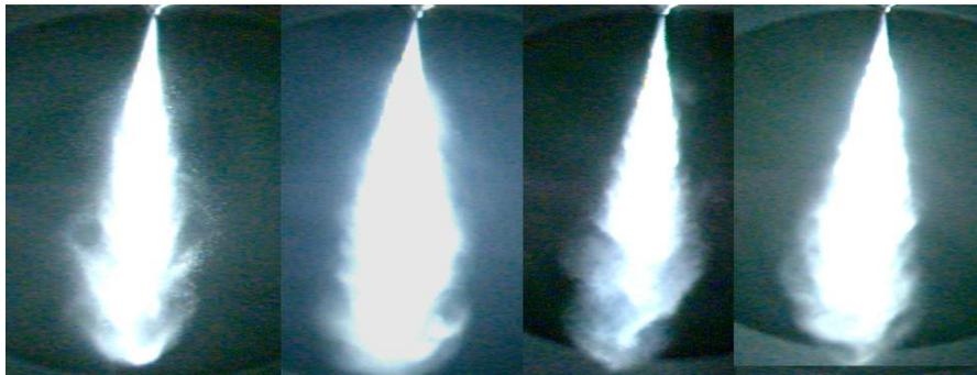
(a) Diesel 15MPa (b) Diesel 100MPa
