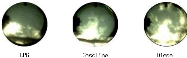
Fig. 3.59 Flames just before termination at trap pressure of 0.4MPa
