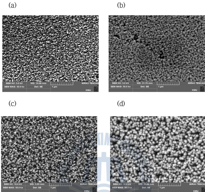
Fig 25. The result of FE-SEM about ZnO nanorods according to temperature at the growth concentration of 0.3 M%
