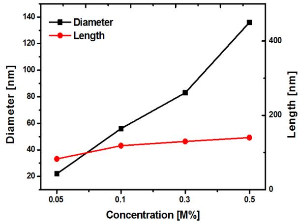
Fig 22. The length and diameter of ZnO nanorods according to concentration at 90°C
