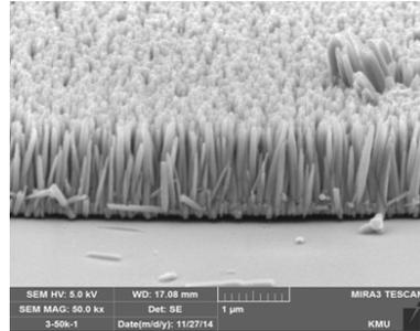
Fig 20. The effect of ZnO seed layer when grown the ZnO nanorods
