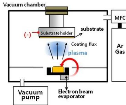
Fig 12. General methods of Ion plating system
