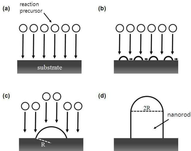
Fig 3. Schematic illustrating VS nanowire growth mechanism including four stages: (a) reaction precursor, (b) cluster migration, (c) nucleation on substrate surface, (d) anisotropic 1-D growth of nanorods.
