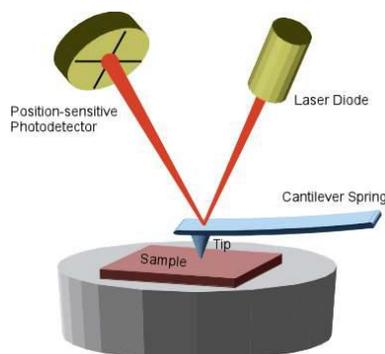
Fig 17. A schematic describing the operation of the AFM
