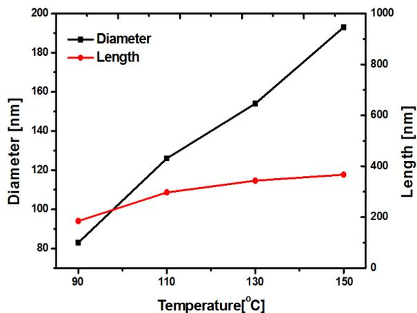
Fig 26. The length and diameter of ZnO nanorods according to temperature at 0.3 M%
