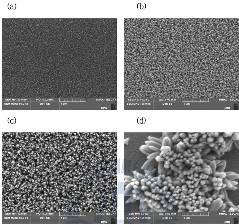
Fig 21. The result of FE-SEM about ZnO nanorods according to concentration at the growth temperature of 90°C
