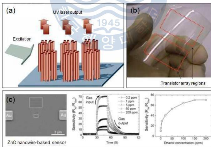
Fig 7. The application of ZnO nanorods and nanowire (a) Nano laser, (b) transparent flexible transistor, and (c) nano sensor.
