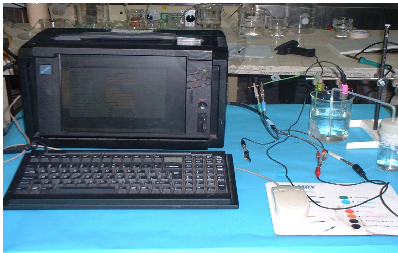
Fig. 3.5 Photograph of potentiostat apparatus
