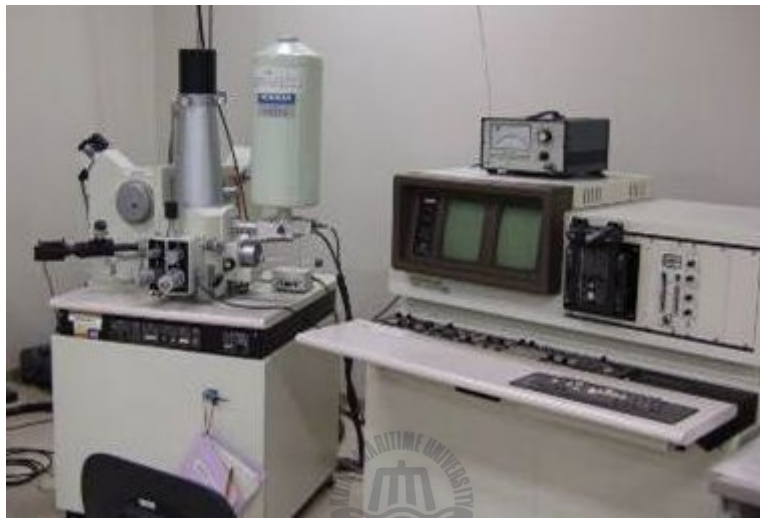
Fig. 3.2 Photograph of scanning electron microscope apparatus
