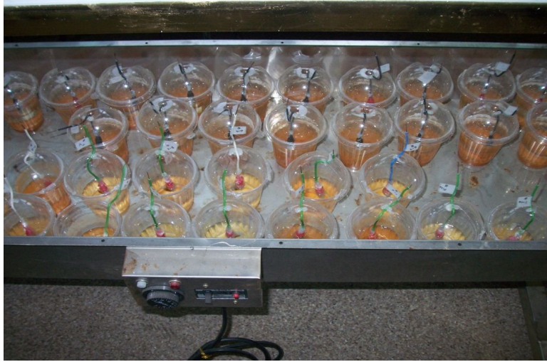
Fig. 3.7 Experimental photographs of corrosion potential measuring in 3% NaCl solution
