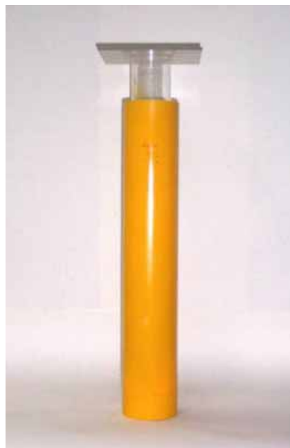
Photo 3.1 Model for Experiment of Wave Exciting Force
