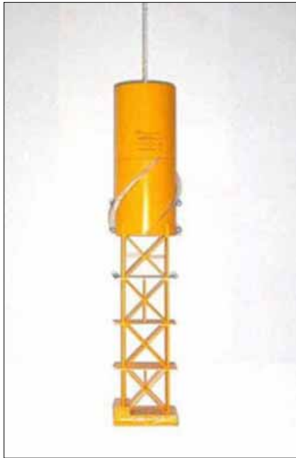
Photo 3.2 Truss Spar Model with & without Strakes for Motion Response test, Scale of 1:400
