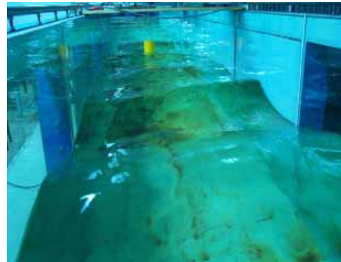
Photo 3.7 Classic Spar Model Test in Irregular Waves
