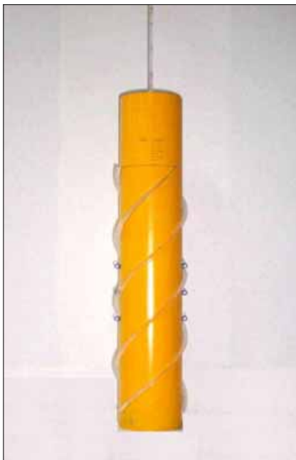
Photo 3.3 Classic Spar Model with & without Strakes for Motion Response test, Scale of 1:400
