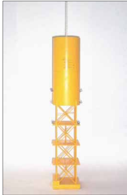
Photo 3.2 Truss Spar Model with & without Strakes for Motion Response test, Scale of 1:400
