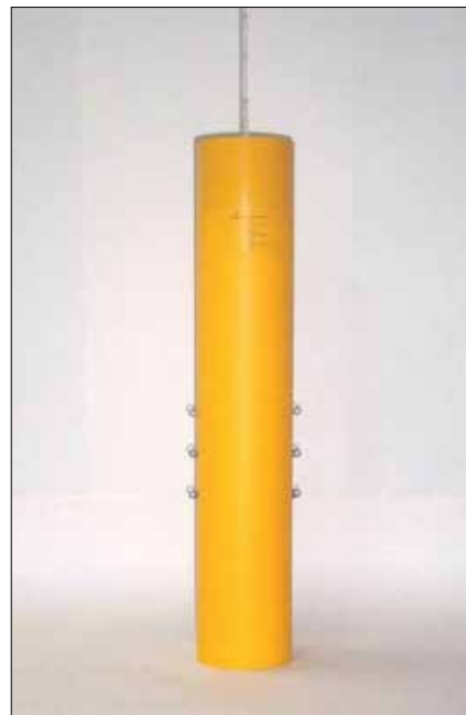
Photo 3.3 Classic Spar Model with & without Strakes for Motion Response test, Scale of 1:400
