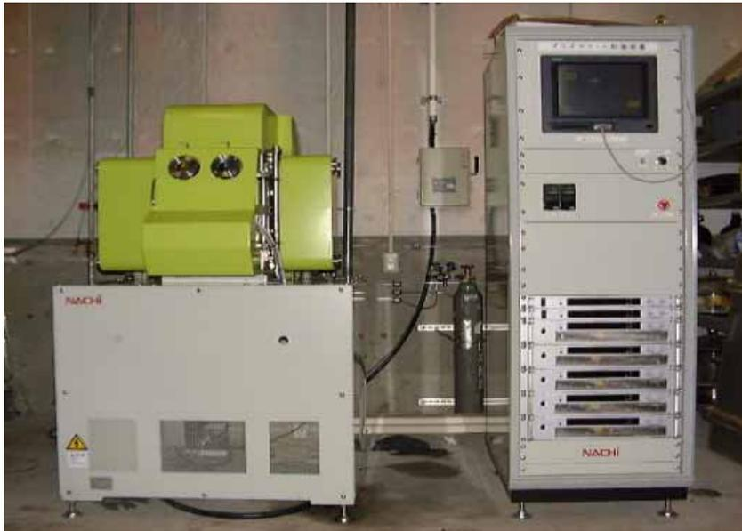
Fig. 3.1 The inclination opposite target type DC magnetron sputtering equipment
