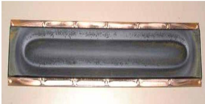
Fig. 3.4 Shape of used Target
