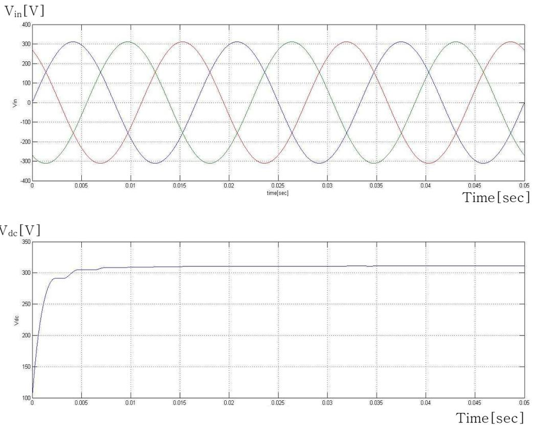
Fig. 4.43 Voltage waveform of power source(Y-connected)
