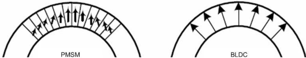
Fig. 3.5 Flux density of permanent magnet motor
