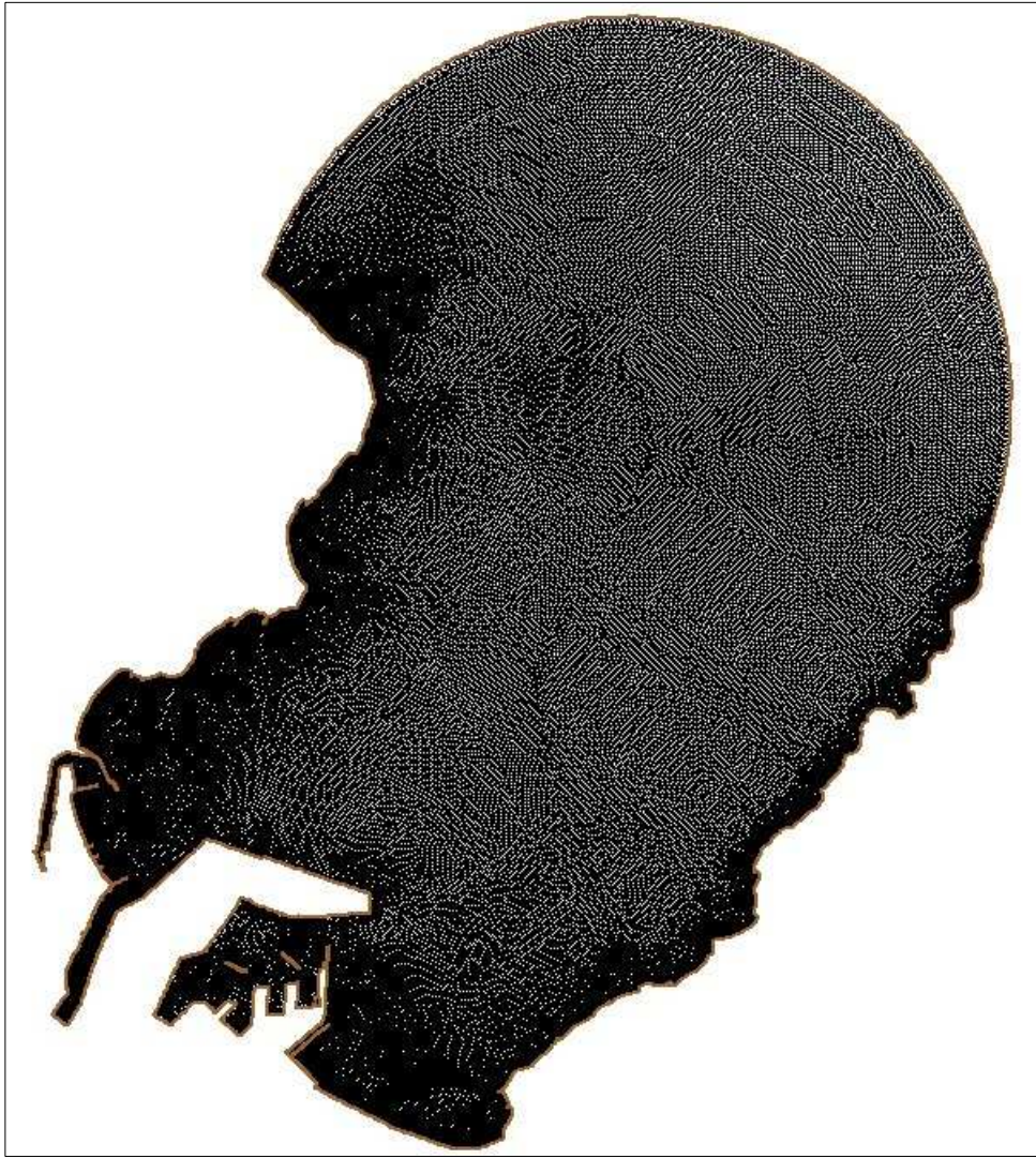
Fig. 4.3 Generated finite element mesh for study area. before construction of New Port in Yeongil Bay
