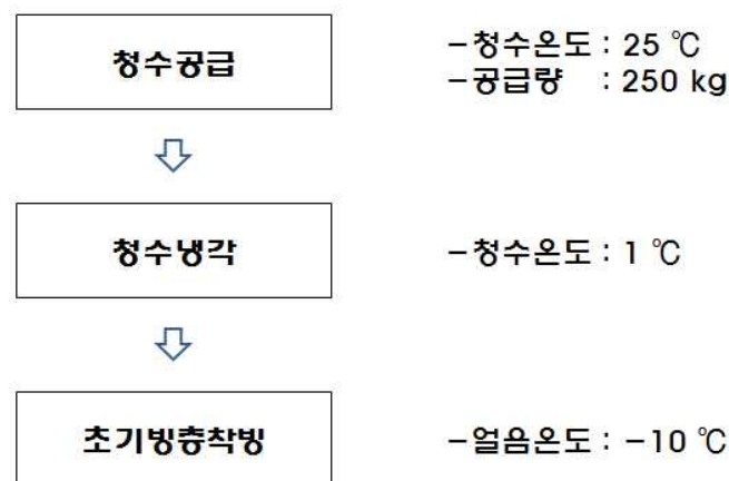
Fig. 3.4 Ice-lining freezing procedure
