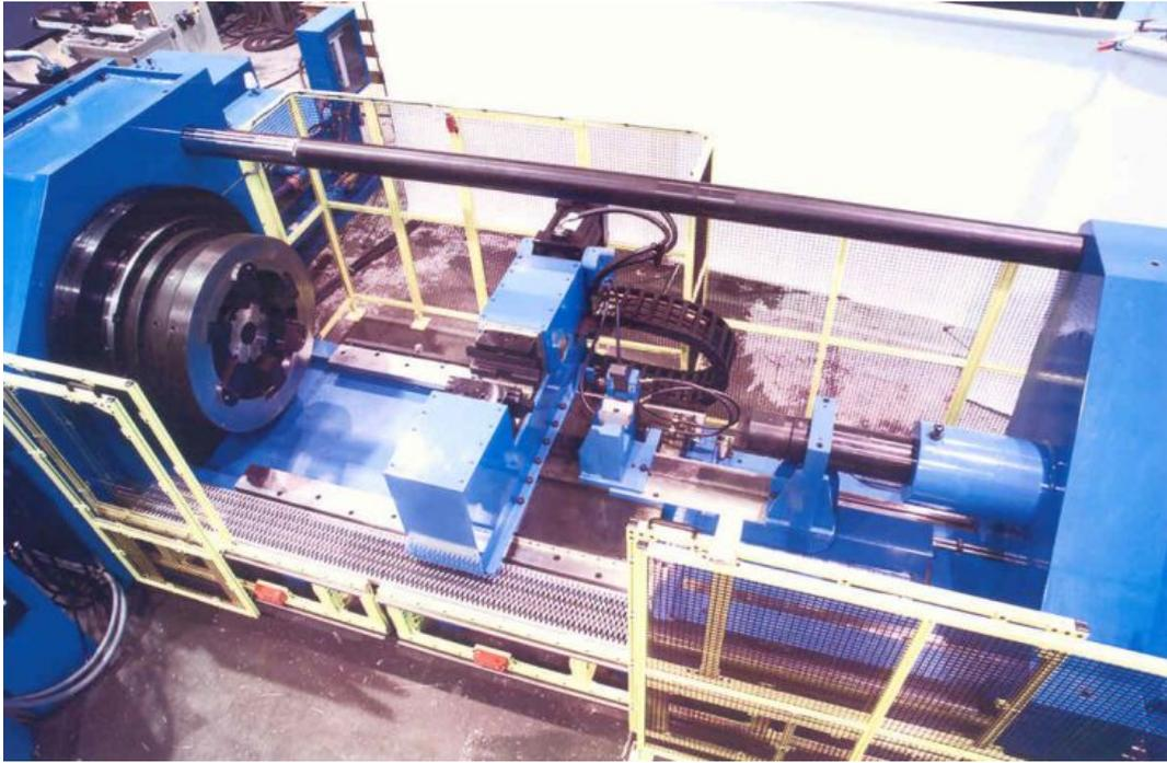
Fig. 17 Inertia friction welding machine
