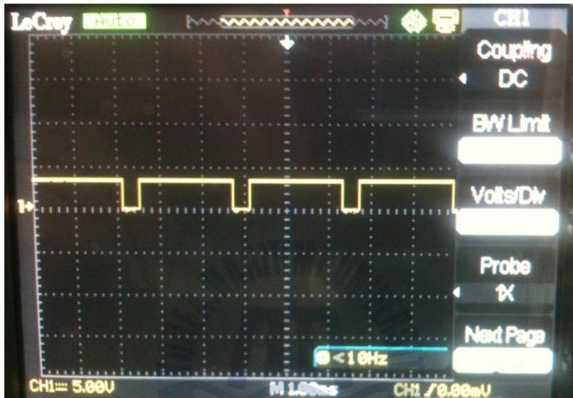
Fig.3.5 The duty rate of PWM on Oscilloscope
