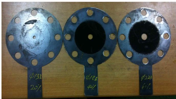
Fig. 3.2 Opening rate adjustment plates at exhaust pipe exit
