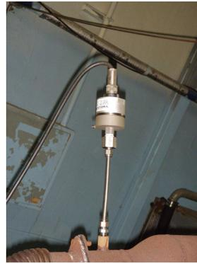
(Exhaust pressure measuring position)
