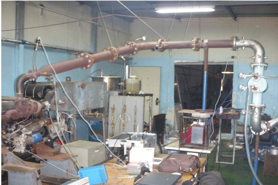
Fig. 5.8 Entire experimental II (installed plate heat exchanger)
