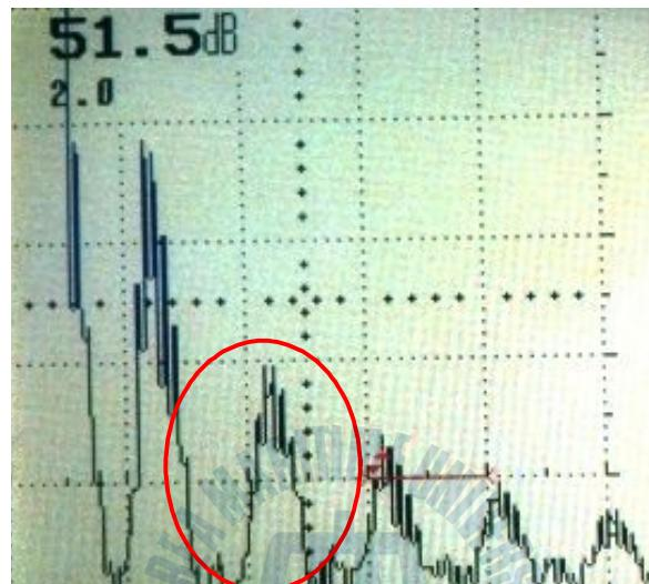
Fig. 4.21 Reflected echo of straight beam from bottom
