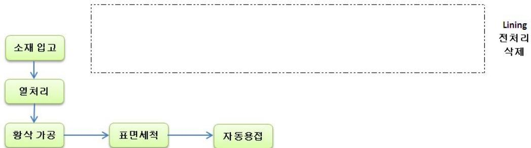
Fig. 3.2 Process flow of auto-welding
