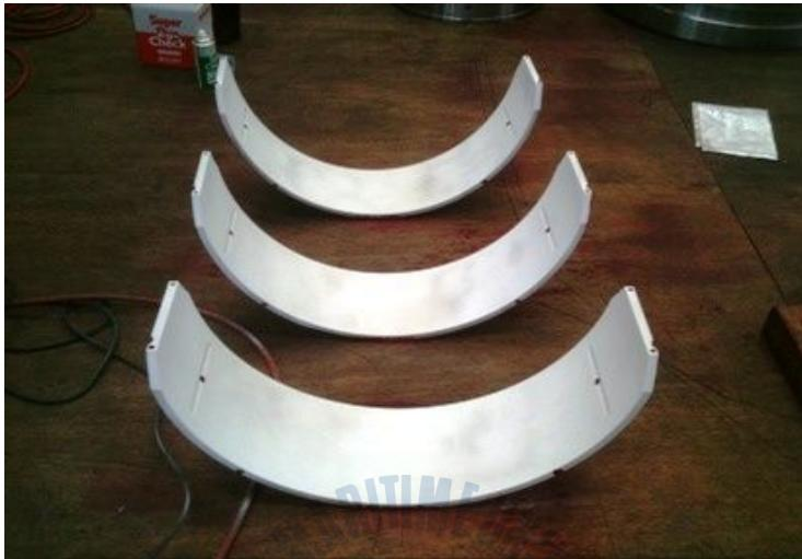
Fig. 3.12 Penetrate testing
