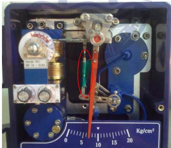
Fig. 4.6 Temperature controller of jacket cooling water cooler (S8000)
