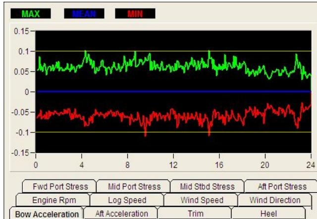
Figure 3.16 Vertical Acceleration ( 2006. 5. 10 )
