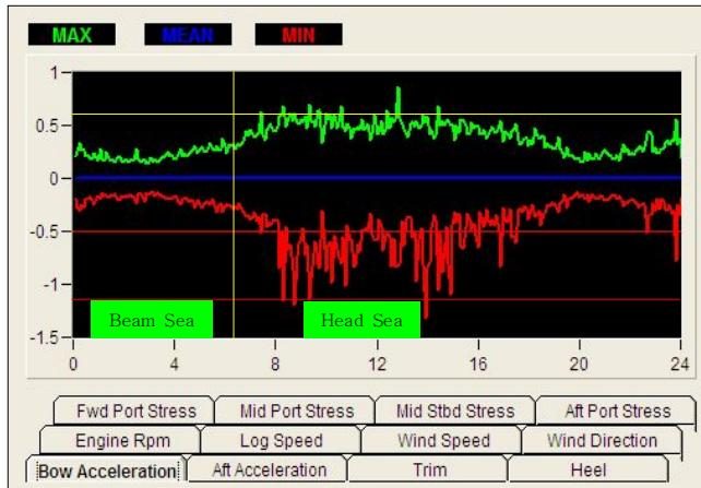
Figure 3.31 Vertical Acceleration ( 2006. 6. 3 )
