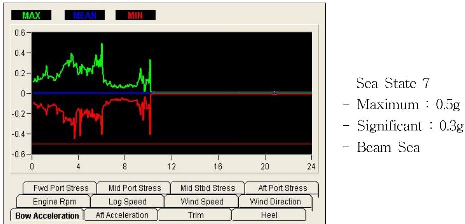
Figure 3.33 V. Acceleration (Coastal, 2006. 4. 20)
