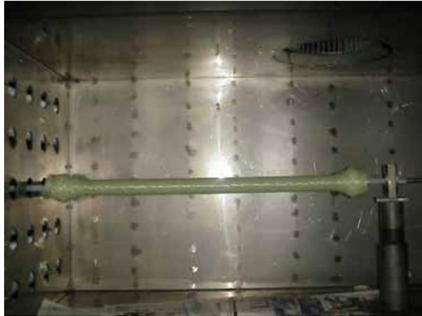
Fig. 19 Photograph of curing in curing oven.
