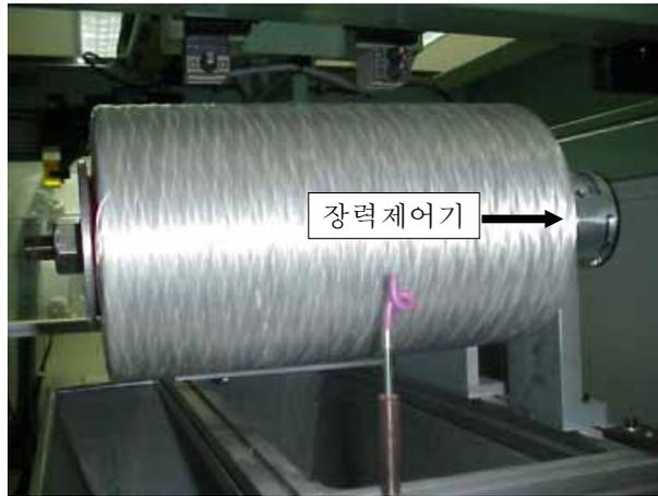
Fig. 15 Photograph of tension control.
