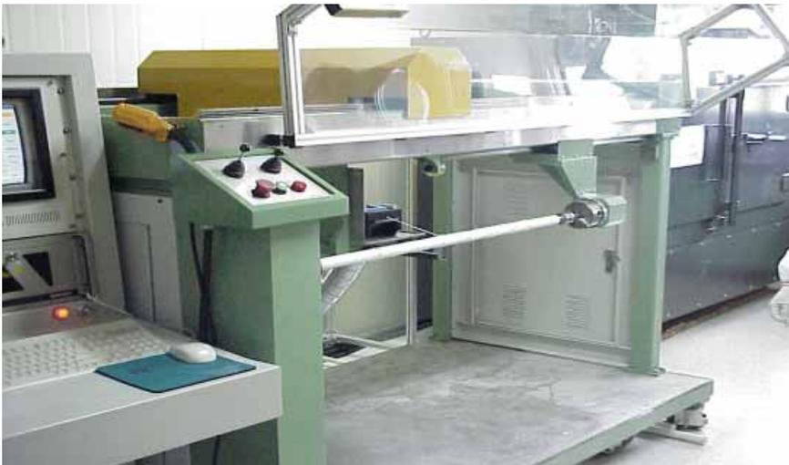
Fig. 13 Photograph of filament winding machine.
