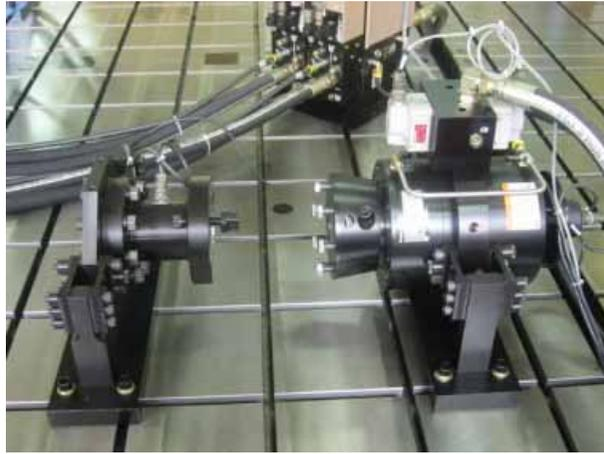
Fig. 30 Photograph of torsional test machine.
