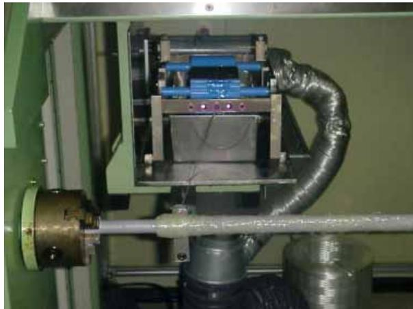
**Fig. 18 Photograph of filament winding.**
