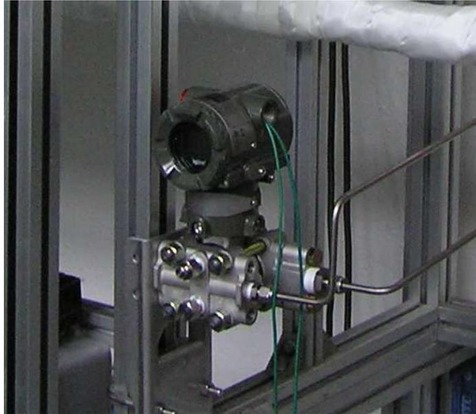
Fig. 3.9 Photograph of pressure drop transmitter
