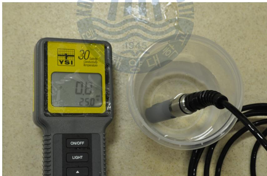
Fig. 2-37 Salinity Measurement of Sea Ice
