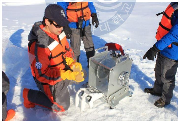
**Fig. 2-34** 19cm Sea Ice Core Sample Cut with the Cutting Machine
