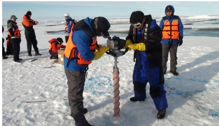
Fig. 2-29 Coring with 3-inch Diameter Kovacs Corer
