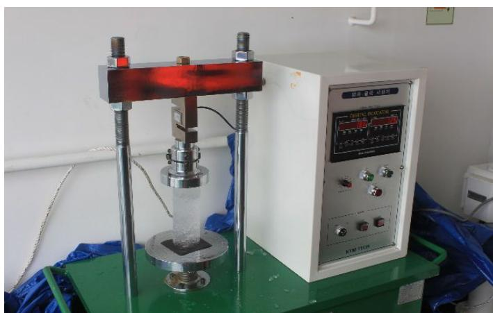
Fig. 2-21 Uniaxial Compression Tester
