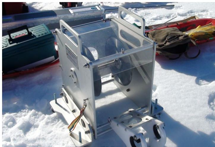
**Fig. 2-33** Sea Ice Core Sample Cutting Machine
