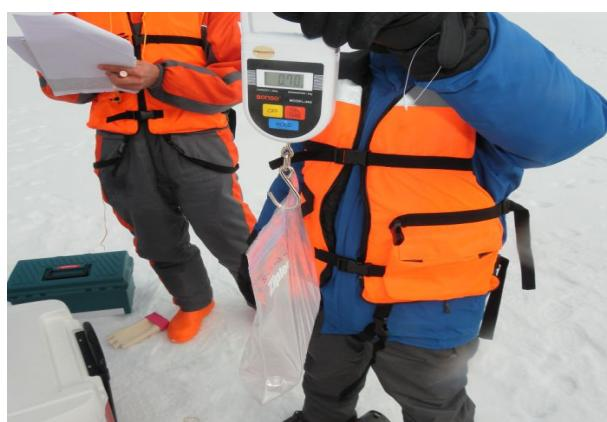
Fig. 2-32 Sea Ice Weight Measurement
