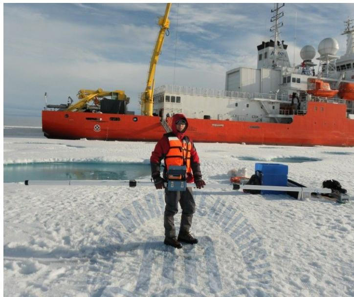
**Fig. 2-27** Ice Thickness Measurement using an Electromagnetic Induction Sensor(EM31)
