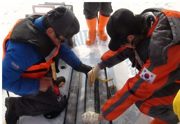
Fig. 2-31 Sea Ice Temperature Measurement using Probe Type Thermometer
