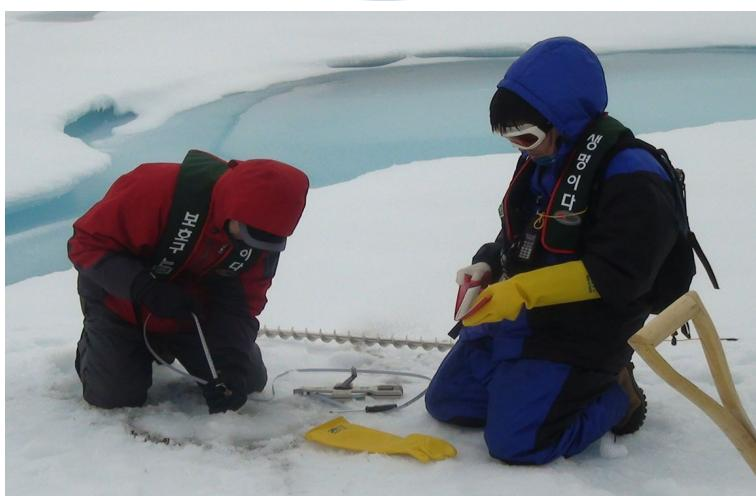
Fig. 2-26 Ice Thickness Measurement with Tape Measure
