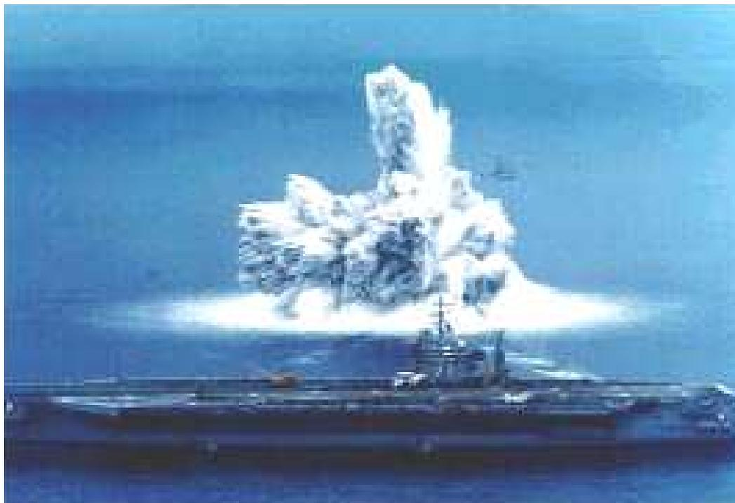
**Fig. 2.8** Underwater explosion for full-scale shock test
