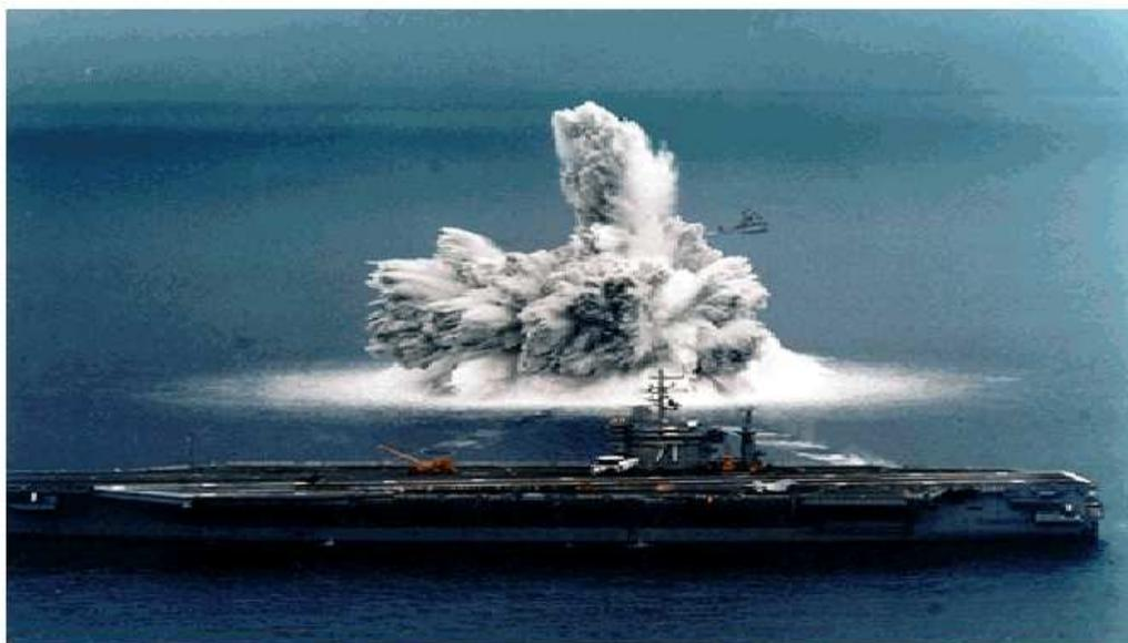
Fig. 3.5 Ship shock trial
