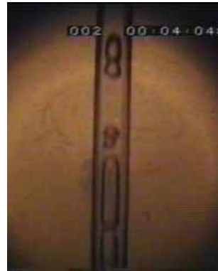
(b) Slug flow ( j_l = 0.796 \text{ m/sec} , j_g = 0.140 \text{ m/sec} )
