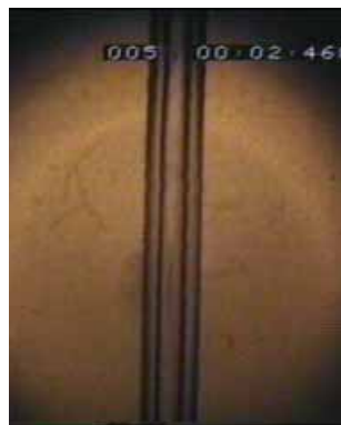
(d) Annular flow ( j_l = 0.796 \text{ m/sec} , j_g = 0.562 \text{ m/sec} )
