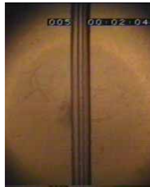
(d) Annular flow ( j_l = 0.531 \text{ m/sec} , j_g = 2.246 \text{ m/sec} )
