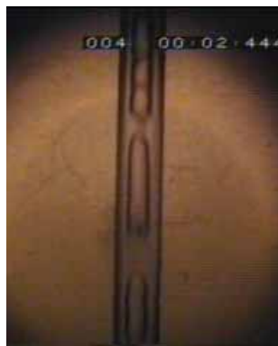
(c) Churn flow ( j_l = 0.796 \text{ m/sec} , j_g = 0.421 \text{ m/sec} )
