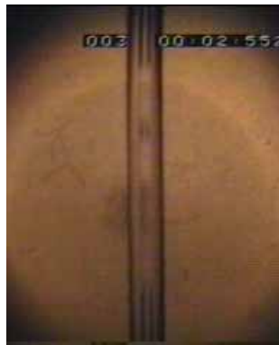
(c) Churn flow ( j_l = 0.531 \text{ m/sec} , j_g = 1.123 \text{ m/sec} )
