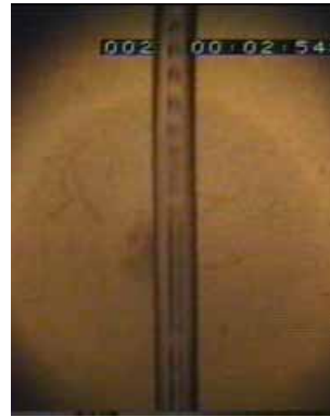
(b) Slug flow ( j_l = 0.531 \text{ m/sec} , j_g = 0.562 \text{ m/sec} )
