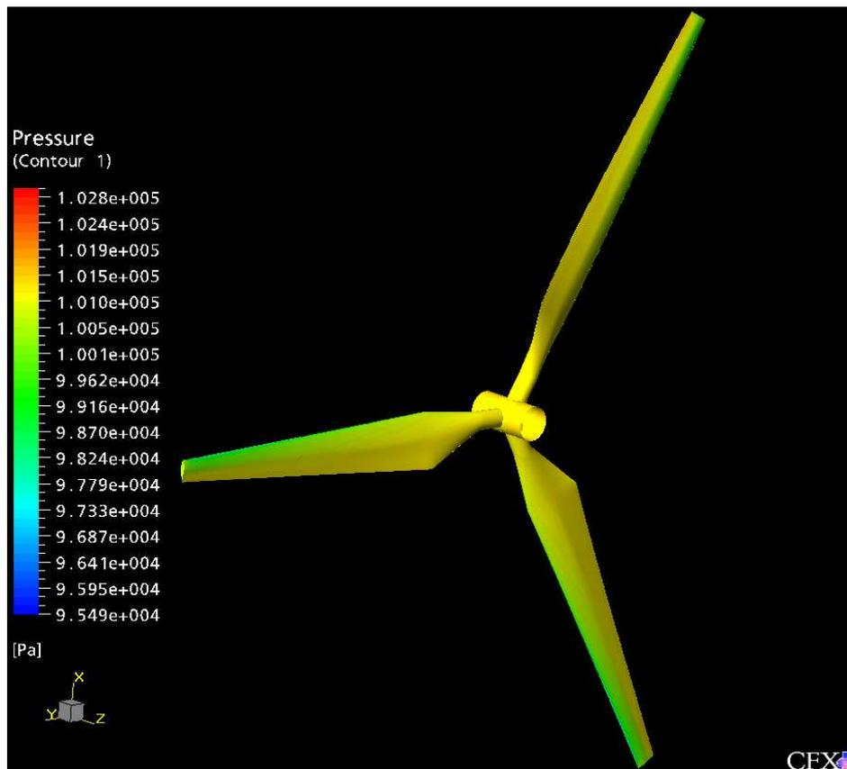
Fig. 5.24 Suction side surface pressure distribution
