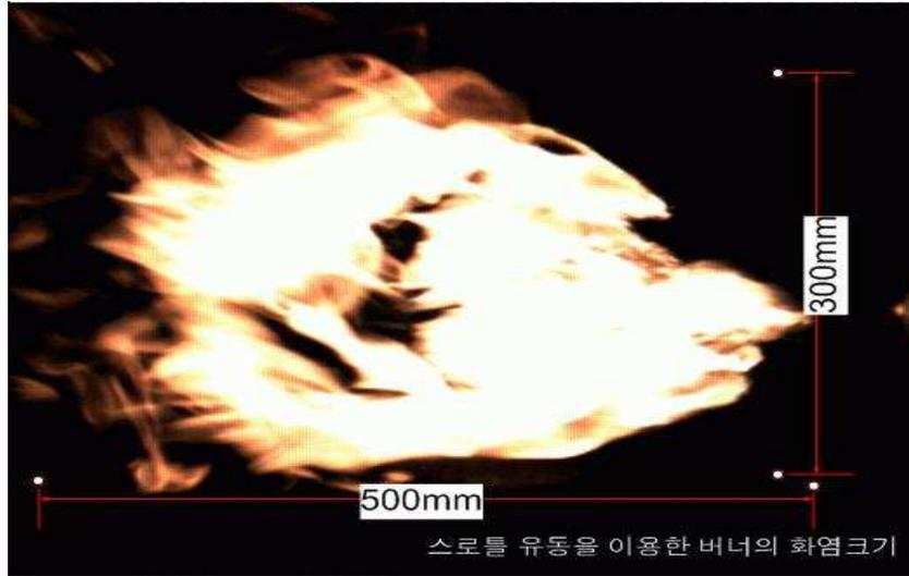
FIG. 4.2 Dimensions of swirl burner flame
