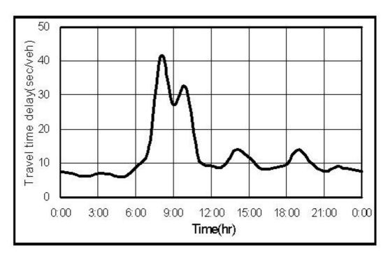
Fig 2.8 Average Delay distribution (Inbound)
