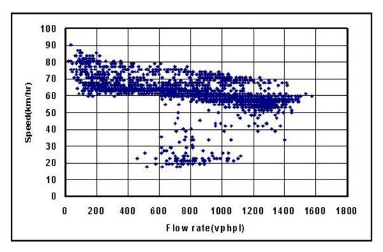
Fig 2.10 Relationship between speed and flow rate
