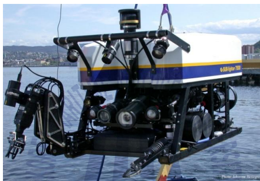
Fig.1.3: A typical Remotely Operated Vehicle
