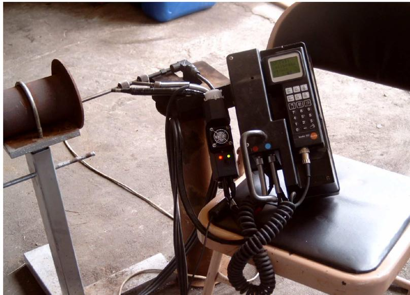
Fig. 3.3 Engine exhaust gas instrument
