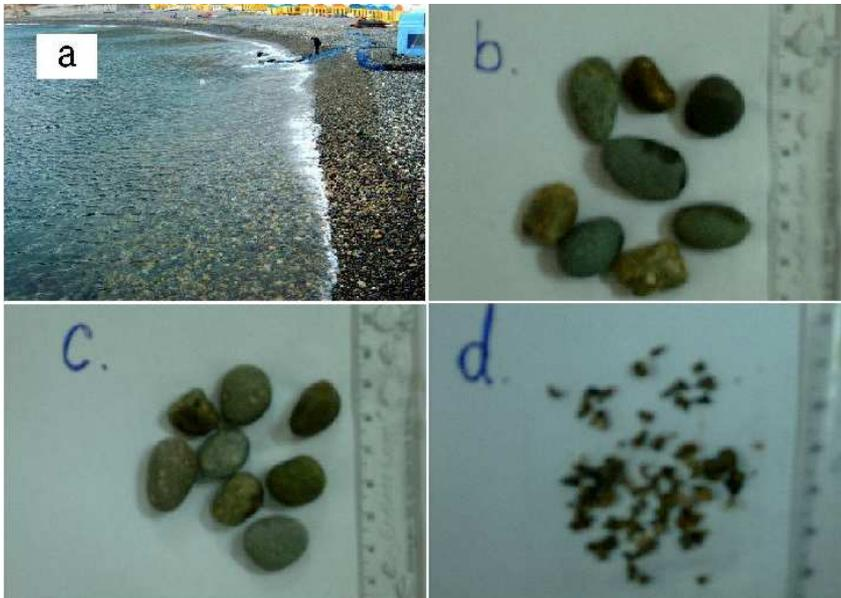
Fig. 3.2 Photographs of the gravels used for the biological activity tests((b) upper ; (c) middle and (d) bottom parts)
