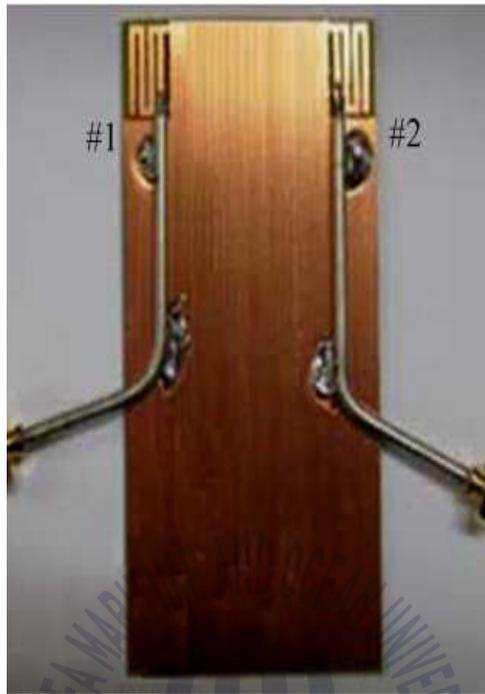
Fig. 2-17 Photograph of fabricated reference antenna.
