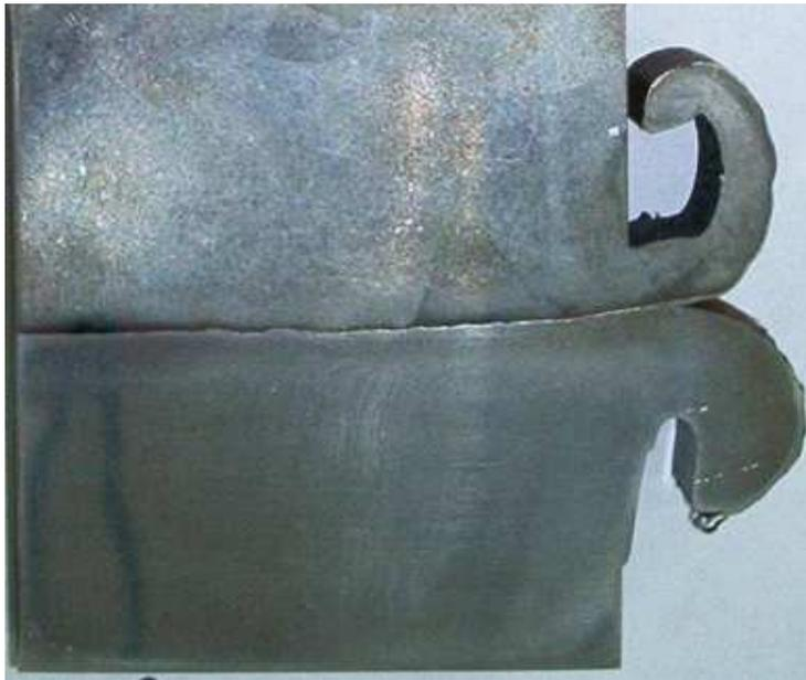
(b) cross section shape for welded joint
