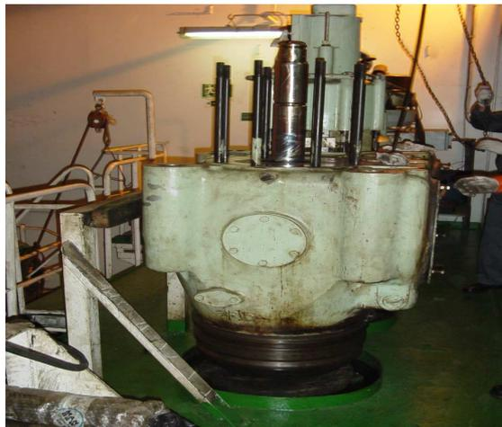
Photo 15. Valve bottom piece and valve are assembled with exhaust valve housing.
