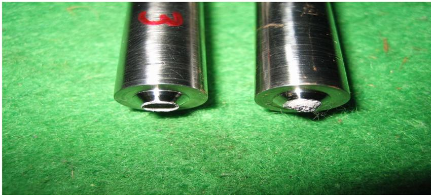
photo 11 View of notched area of broken tensile specimen
