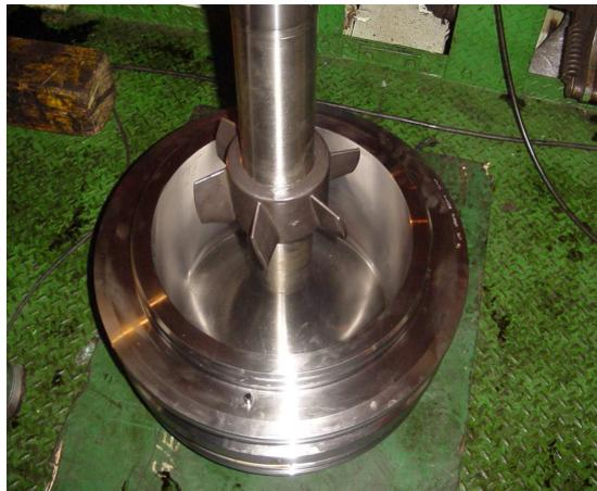
Photo 14. Valve bottom piece and valve are assembled
