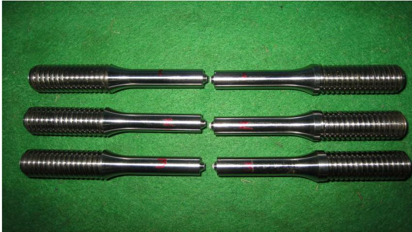
photo 10 Broken notched tensile specimens
