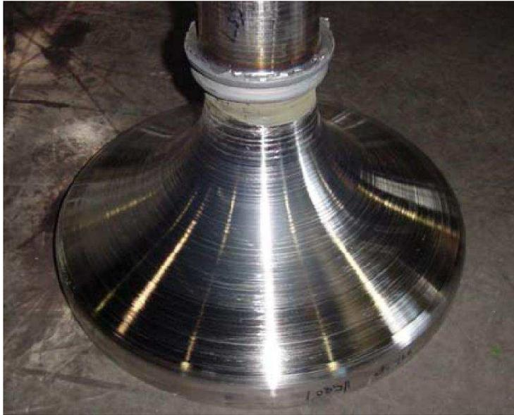
(a) friction welded exhaust valve product
