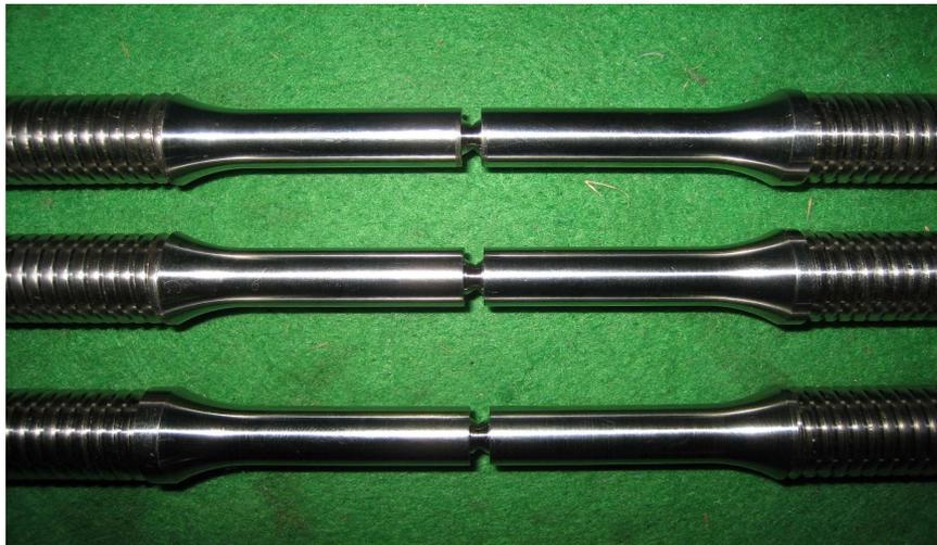
photo 9 Notched tensile test specimens ready for test.
