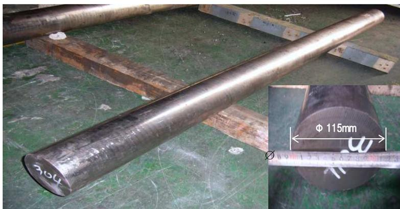
(b) stem part shape of exhaust valve ( 115mm)
