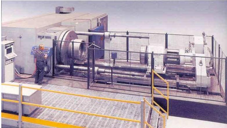
Photo 1 Appearance of Inertia friction welding machine
