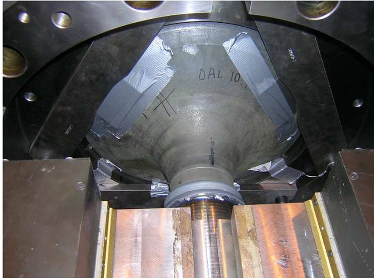
(e) Head and stem part on phase of friction welding
