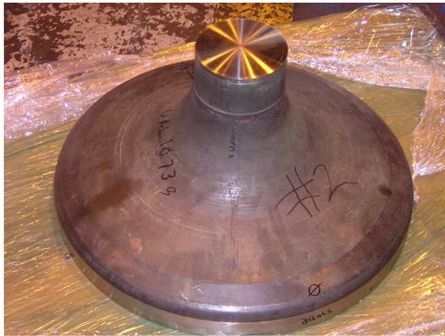
(a) head part shape of exhaust valve ( 115mm)
